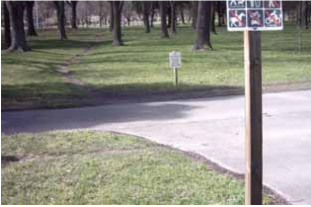
Figure 4: Desire line showing missing path link
